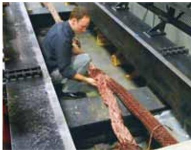
The Samson Advantage includes residual strength testing as a part of the retirement guidelines for the safety of your rope.
